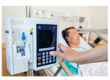
Control panels based on membrane switches in medical environments.
